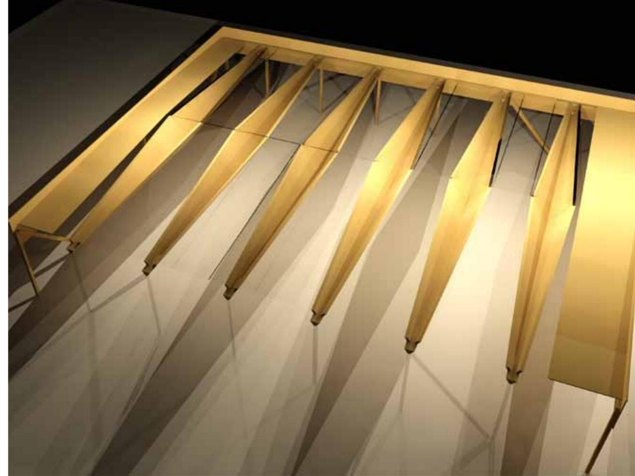
Another structural design concept where KLH® - CLT fits particularly well are thin-walled structures: again, a form of folded plate elements. Extending ship and airplane structural design concepts to architecture, and/or applying the principles of hollow thin-walled profiles' stress-strain behaviour, leads to a source of new possibilities. Here, too, many developments in the best traditions of steel and concrete based structural researches prove to be fruitful.
